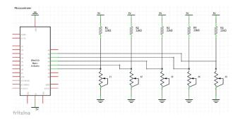
Fig.9.An electrical scheme of the glove.
