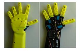
Fig. 5.General view of the 3D printed hand.
