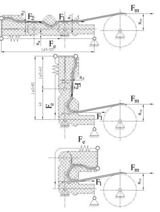
Fig. 7.Stages in the fingers movement and location of the forces.
