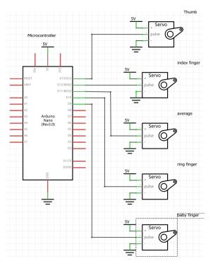
Fig. 8.An electrical scheme of the microprocessor's electrical motion
