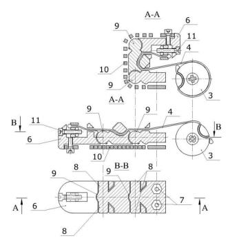
Fig.4. Structure of the hand's fingers.
