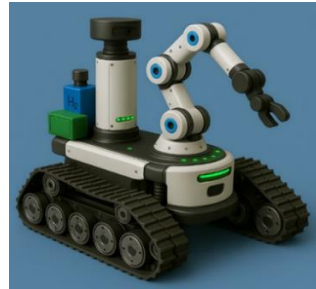
Fig. 7 3D image of a variant of a mobility mechanism with extended chain for a cobot.
