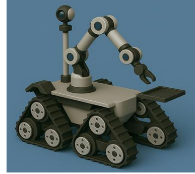
Fig. 5 3D image of a mechanism for mobility with triangular sprockets for a cobot.
