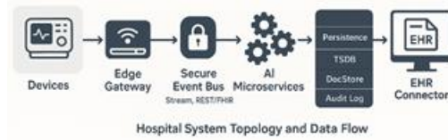
Fig. 2 — System Topology and Data Flow (Edge → Bus → Core → EHR)
