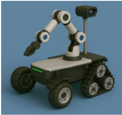
Fig. 9 3D image of a hybrid (mixed) version of a mobility mechanism for a cobot.
