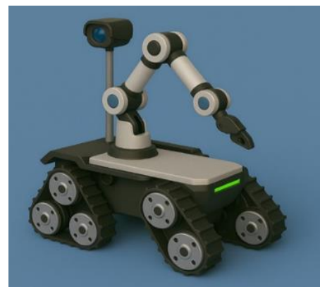
Fig. 8 3D image of a variant of a mechanism for mobility with a combined chain, the first with triangular sprockets and the second with two wheels, for a cobot.
