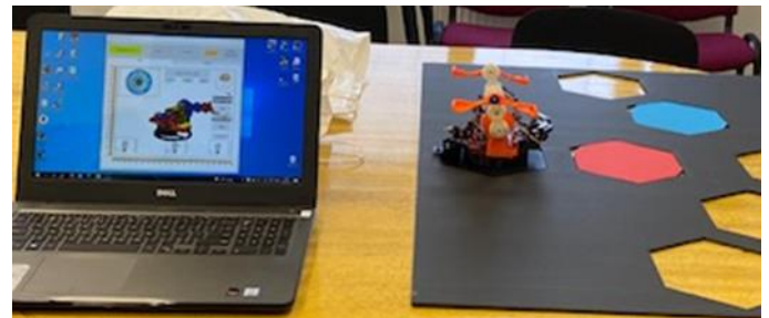
Fig. 2. An interface to control the movement of a walking robot towards a coloured goal.
