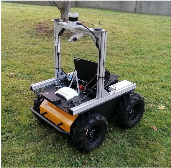
Fig. 4. Laser scanning in indoor and outdoor areas with the Ouster LiDAR OS1 [12].
