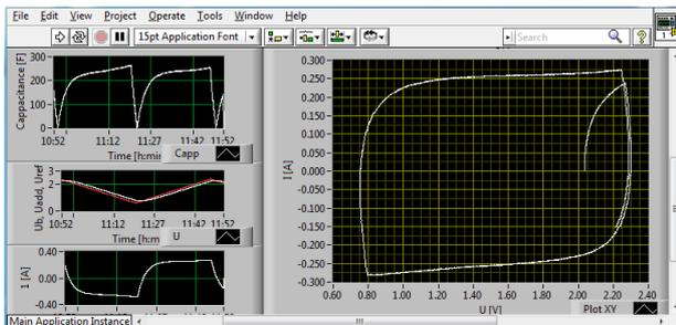
Fig. 1. Supercapacitor cell cyclic voltammetry
