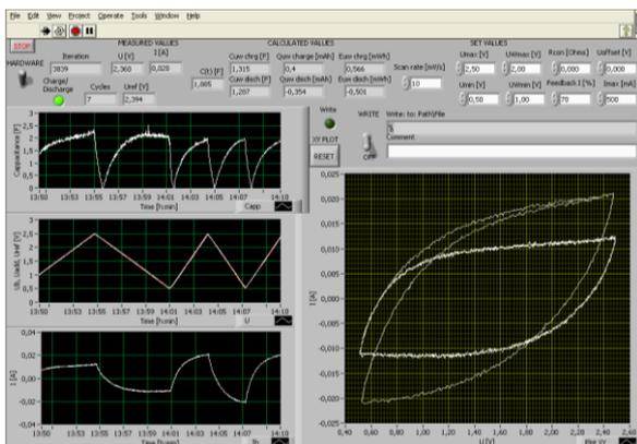
Fig. 2. Asymmetric supercapacitor cell cyclic voltammetry at 5 and 10 mV/s
