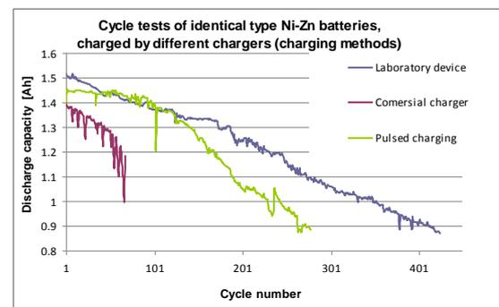
Fig.3 Cycle-life tests of 3 identical Ni-Zn batteries charged by different methods (chargers)
